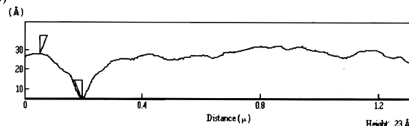
Figure 7. Topography of grafted glass surface from a C 30 -HDPE system after separation: (a) AFM image; (b) height profile
